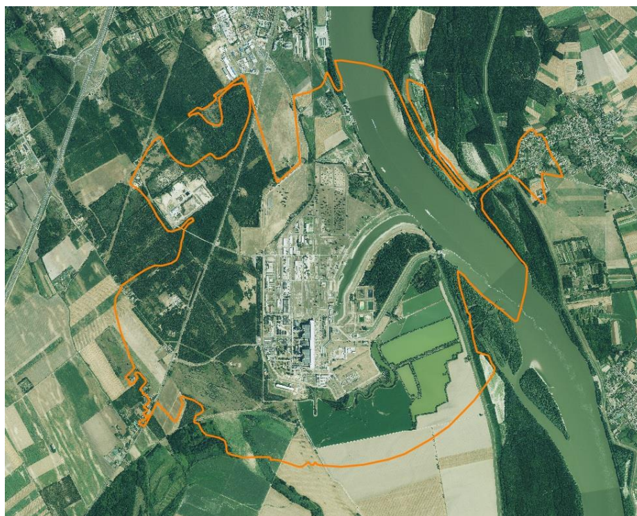
Figure 3.4-1: Cumulative noise impact area for the phases of construction within the operation area
